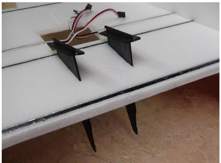
Glue motor mount sides and slotted brackets to wing with Foam-tac.
