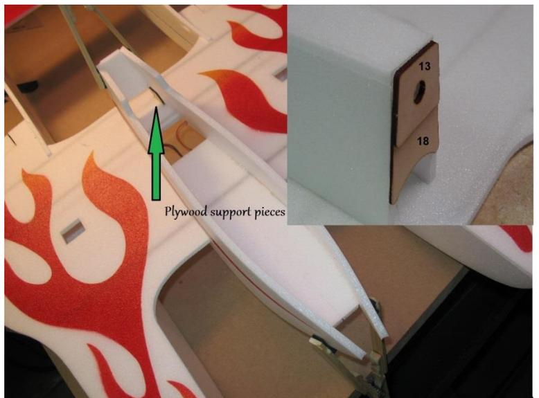
Cut hatch to size and glue top of fuselage in place. **Let glue cure for a few hours before starting the next step.**
