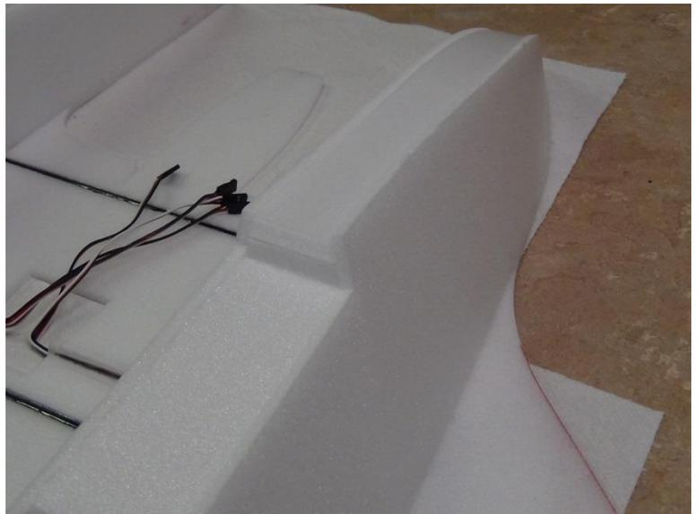
The horizontal stab and carbon trussing can now be glued in place. Make sure sides are straight and square.
