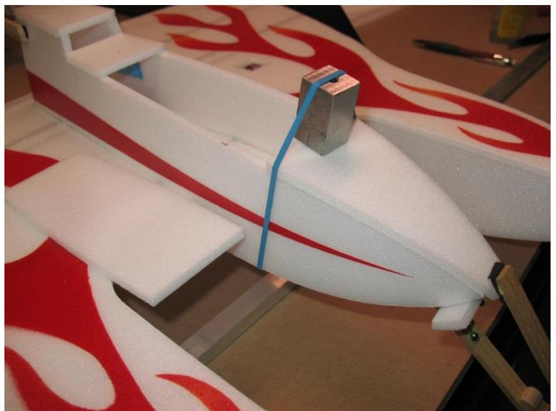
Glue battery support bulk head, and fuselage sides to bottom of wing.
