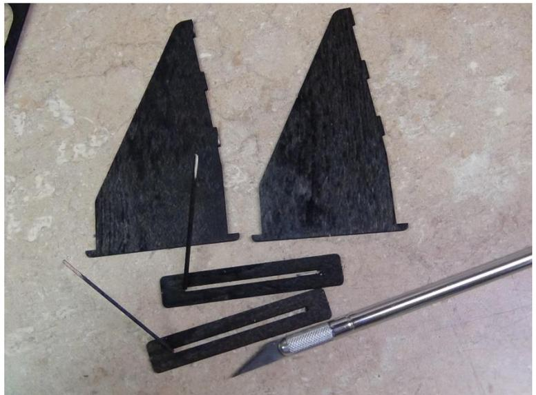
Slide motor mount sides through slotted brackets and into slots in the wing. Note that these are inserted from underneath the wing.
