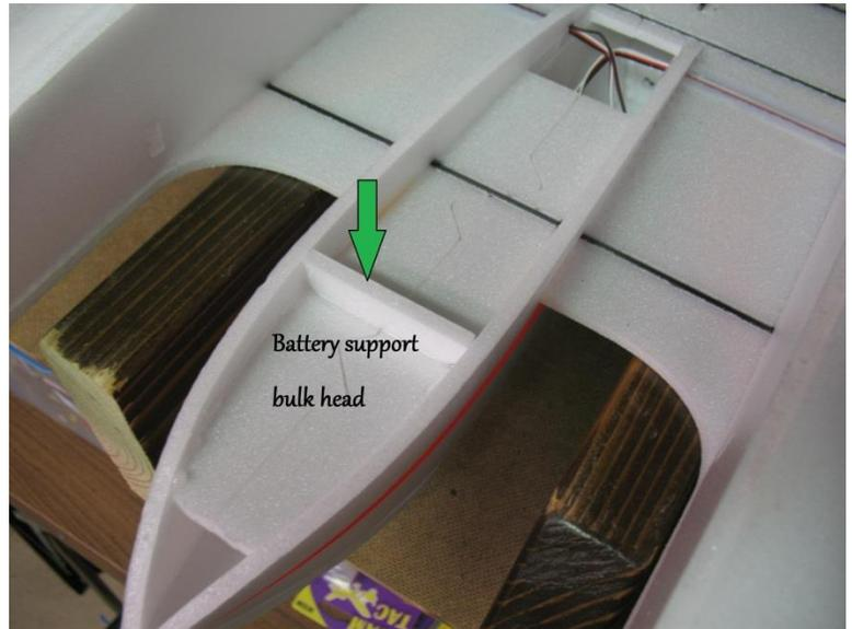
Cut the bottom of the fuselage to size and glue in place. **Let glue cure for a few hours before unclamping.**
