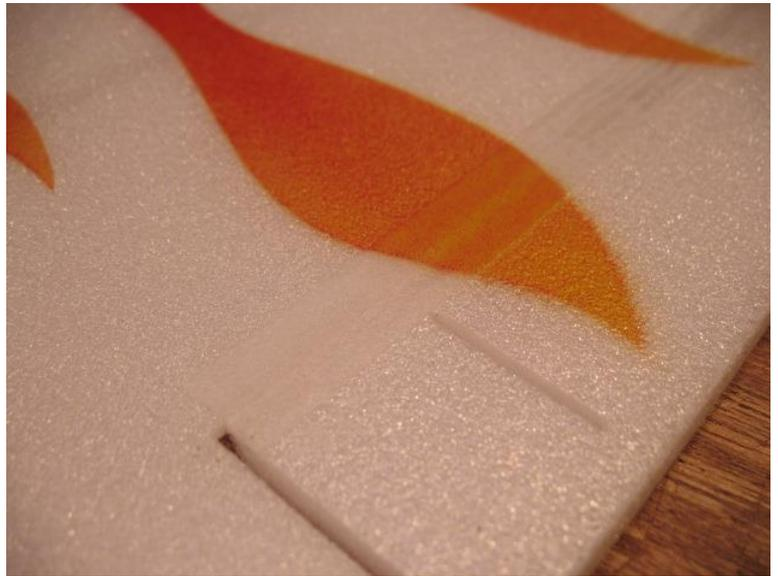
In this photo the servo wire extensions are put into the grooves and covered with Blenderm tape. Note that the wire extensions are kept short near the servo holes, and long at the center to help connect to the receiver.
