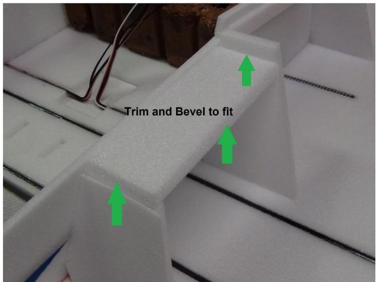
The long front float bottom pieces can now be beveled and trimmed to fit. Gently press and bend the foam on something round like the pipe in the picture.
