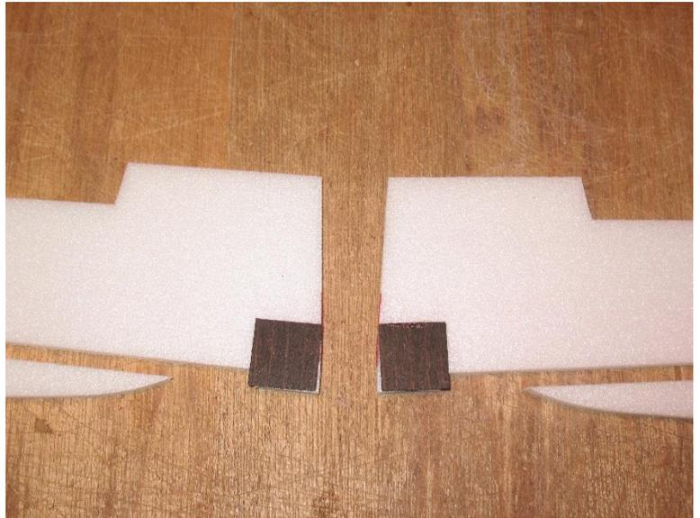
Glue the fuselage sides and plywood support squares to the wing and clamp in place.
