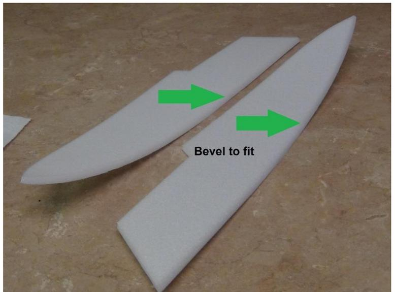
Glue and clamp outer float sides in place. Once they are dried the floats can be trimmed and sanded flat.
