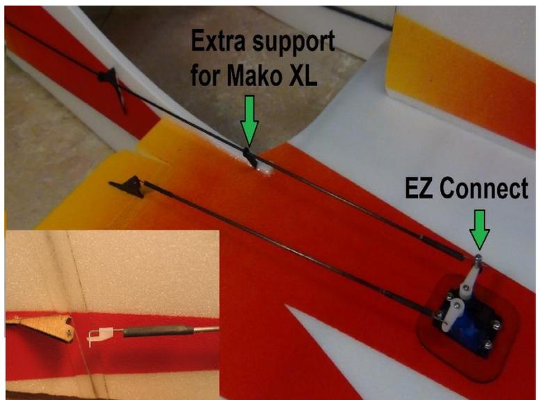
Connect rudders together using a Z bend on one end and a 90 degree bent wire and an EZ link on the other end.
