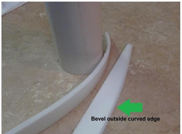
Once float bottoms have been trimmed, beveled, and pre curved. They can be glued in place.
